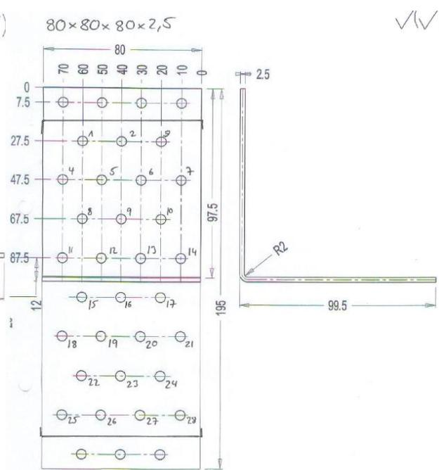
Figure A. 8 Dimensions of angle bracket 80x80x80x2,5
