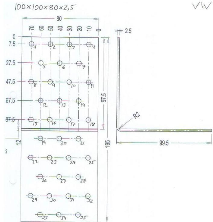
Figure A. 12 Dimensions of angle bracket 100x100x80x2,5
