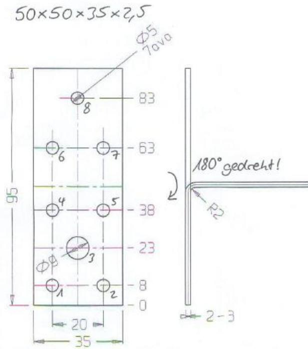
Figure A. 1 Dimensions of angle bracket 50x50x35x2,5
