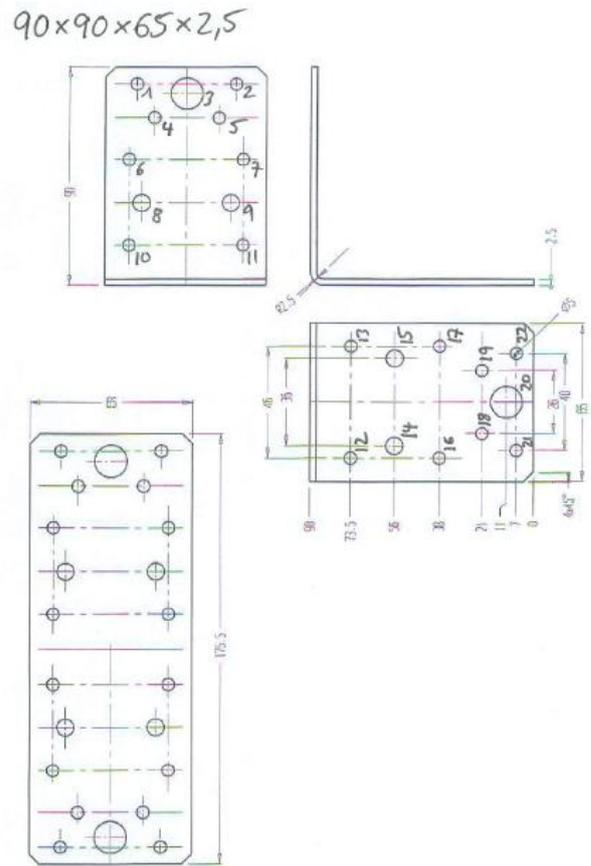
Figure A. 10 Dimensions of angle bracket 90x90x65x2,5
