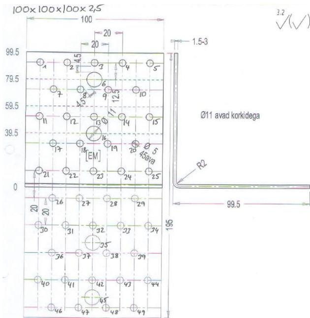
Figure A. 13 Dimensions of angle bracket 100x100x100x2,5
