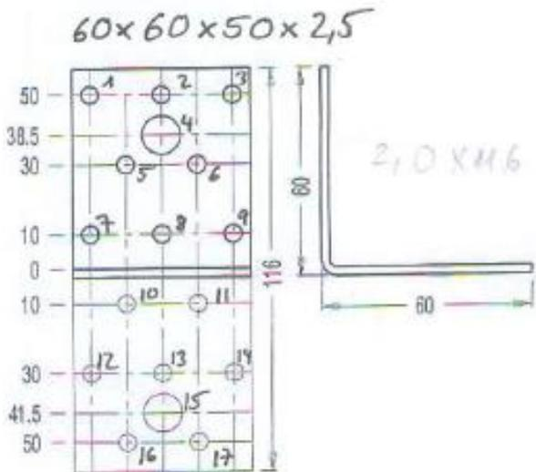
Figure A. 3 Dimensions of angle bracket 60x60x50x2,5
