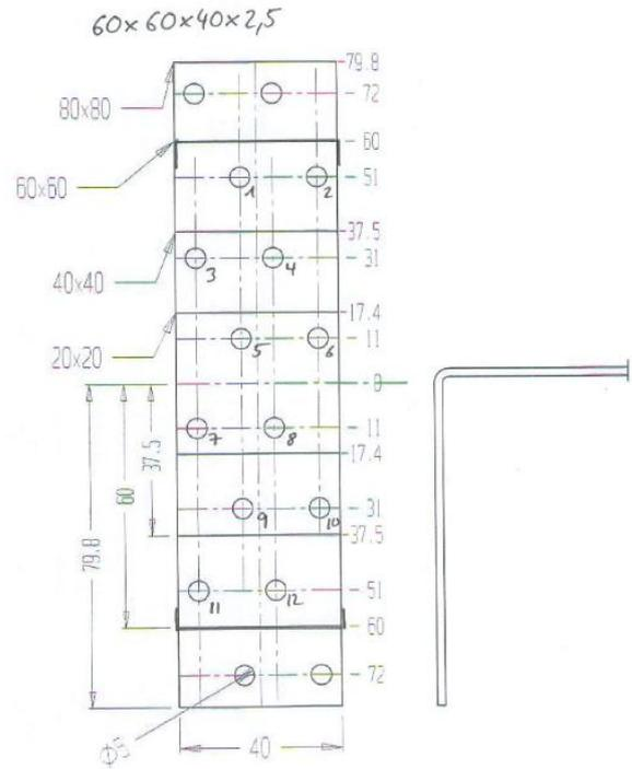
Figure A. 2 Dimensions of angle bracket 60x60x40x2,5
