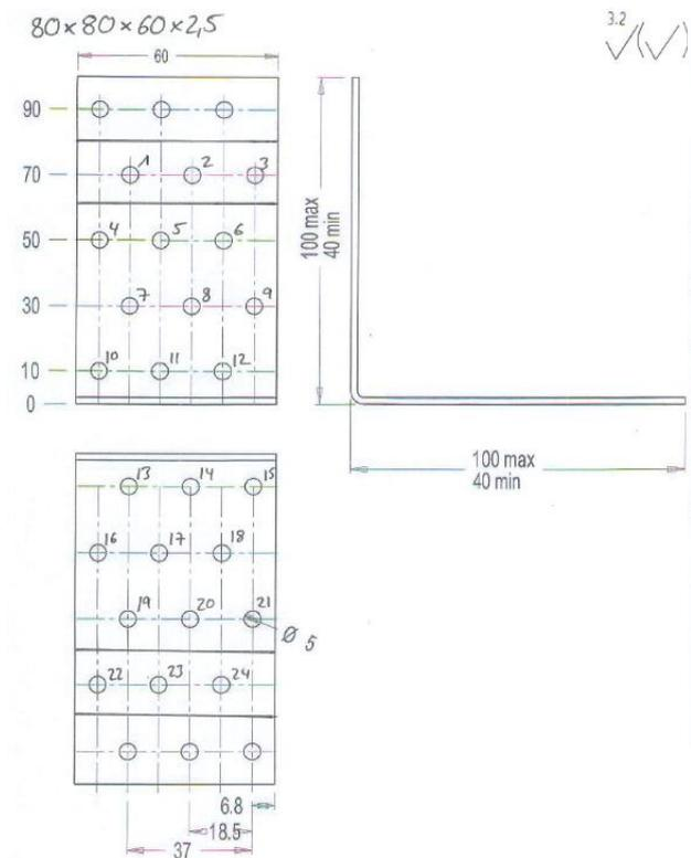
Figure A. 7 Dimensions of angle bracket 80x80x60x2,5
