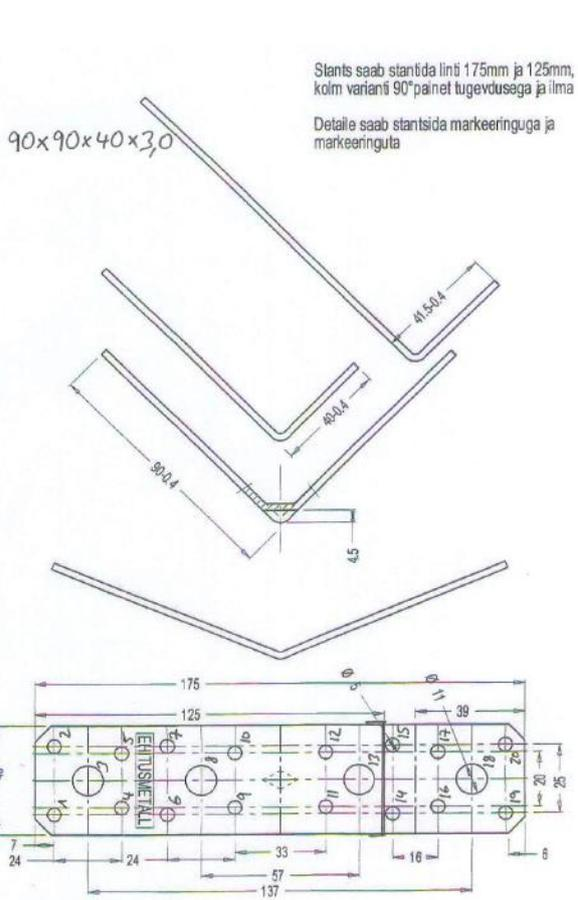
Figure A. 9 Dimensions of angle bracket 90x90x40x3,0
