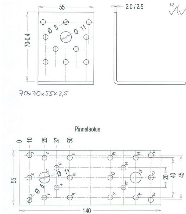
Figure A. 5 Dimensions of angle bracket 70x70x55x2,5
