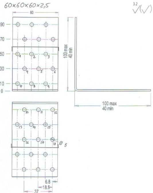
Figure A. 4 Dimensions of angle bracket 60x60x60x2,5
