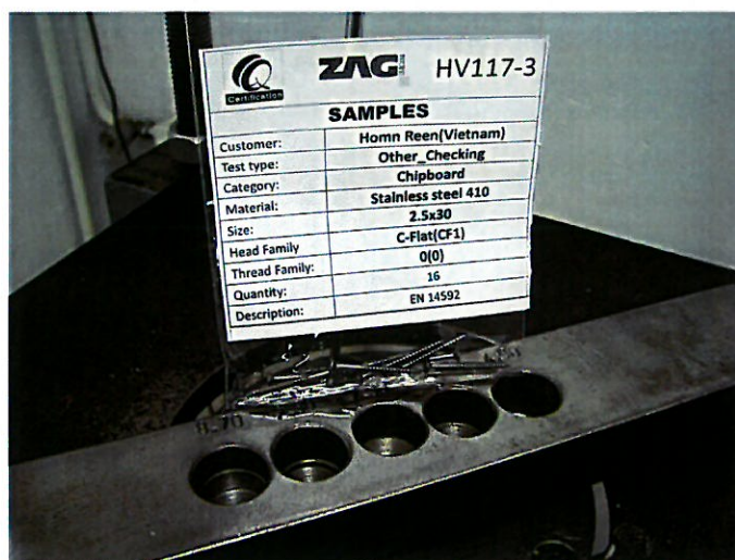
Figure 8: Tensile capacity test – test setup and specimens
