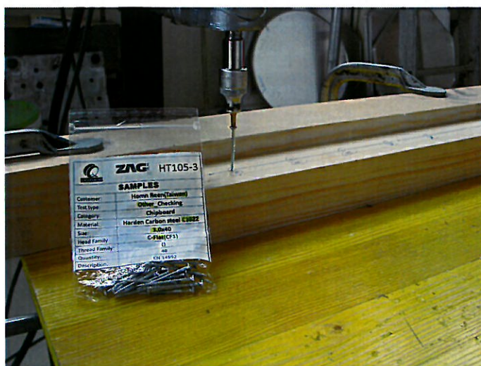
Figure 9: Torsional resistance to insertion of screws – test setup and specimens
