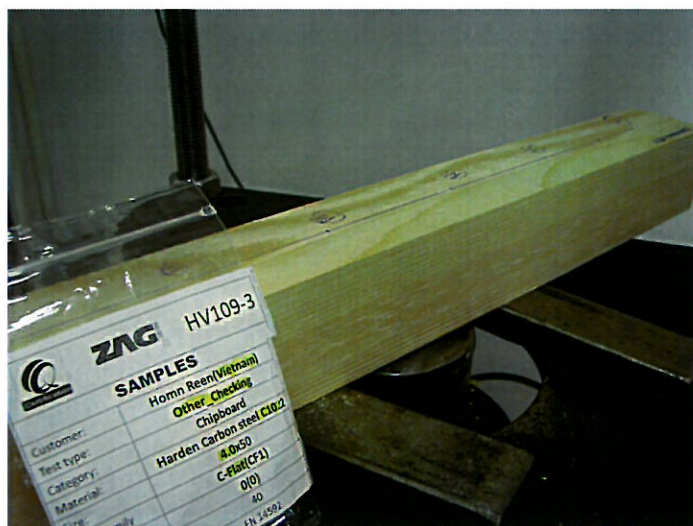
Figure 6: Withdrawal parameter test – test setup and specimens
