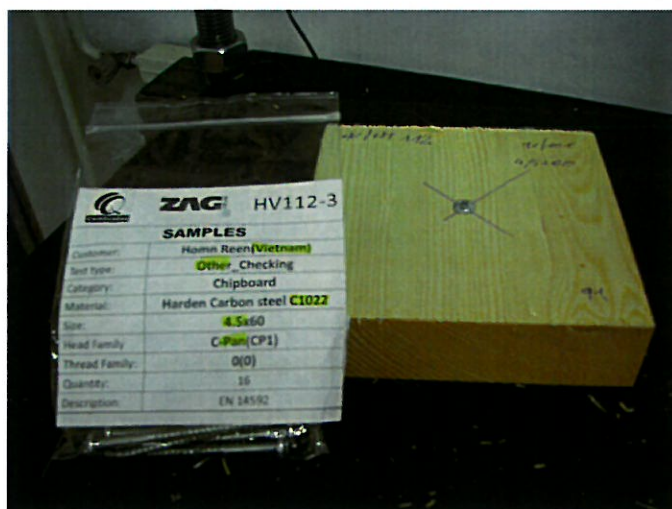
Figure 7: Head pull through test – test setup and specimens
