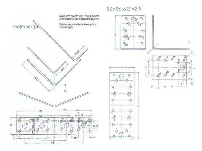
Figure A. 9 Dimensions of angle bracket 90x90x40x3,0
