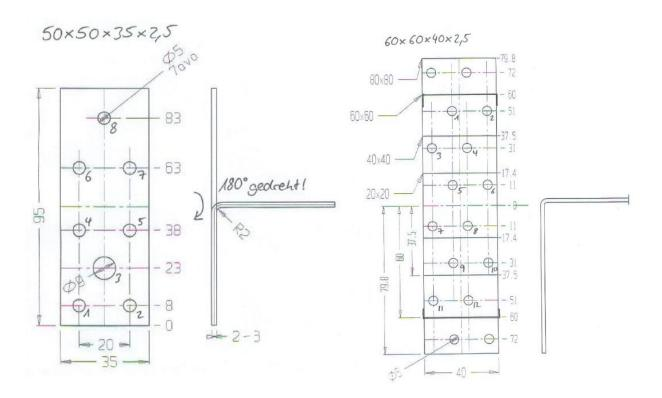
Figure A. 1 Dimensions of angle bracket 50x50x35x2,5
