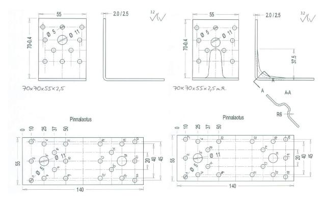
Figure A. 5 Dimensions of angle bracket 70x70x55x2,5
