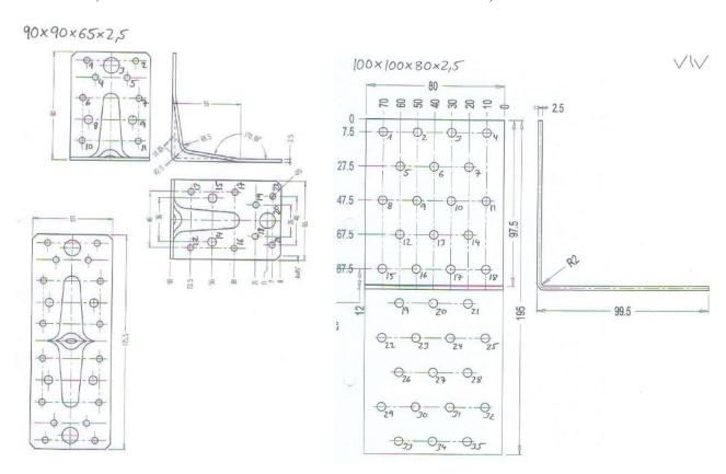
Figure A. 11 Dimensions of angle bracket 90x90x65x2,5(with rib)
