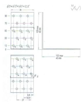
Figure A. 3 Dimensions of angle bracket 60x60x50x2,5
