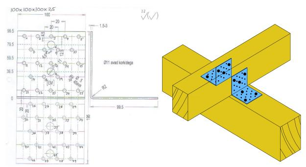
Figure A. 13 Dimensions of angle bracket 100x100x100x2,5
