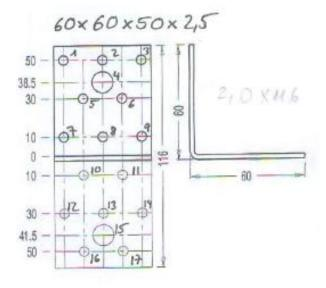
Figure A. 2 Dimensions of angle bracket 60x60x40x2,5
