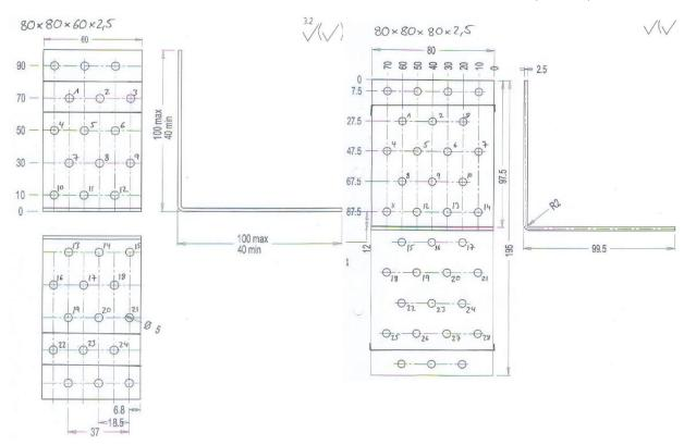
Figure A. 7 Dimensions of angle bracket 80x80x60x2,5
